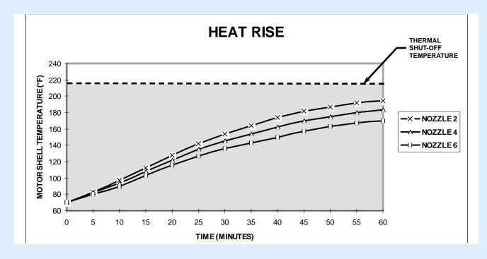
This pump model is in the shaded area of the Performance Data and Heat Rise charts, meaning it is capable of sustaining continual running at any of the above listed pressures, without shutting down to allow the motor to cool. To conserve wearing parts, however, the pump should only operate as needed.
