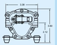
Series 5800 Pump Floor Care Applications 115 VAC Operation 3/8" NPT Female Ports Pressure Switch Set to 170 PSI Internal Pressure Bypass Sealed Motor to Prevent Moisture Intrusion Steel Mounting Plate (Other Types Available)
